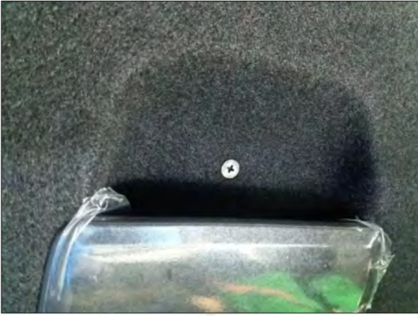
3. Remove the screws and remove the original car back trim panel.
