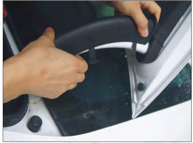
4. Undo the button to remove the trim panel.
