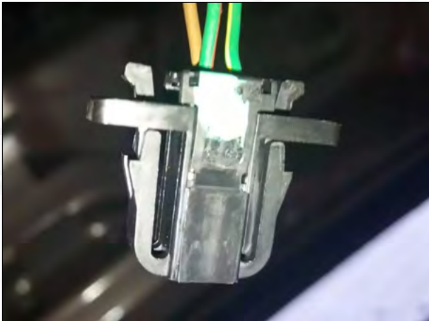
15. Unplug the original car socket in the tailgate lock and plug the three-way socket.
