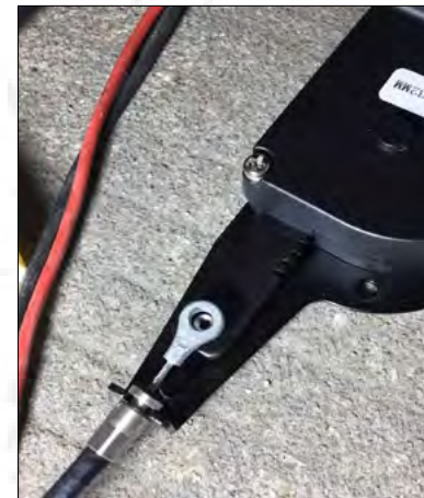
18. Take out the screws of the motor and place the cable on the motor. (As shown in the figure).
