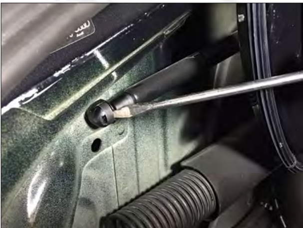
7. Use a flat-blade screwdriver to pry the original car spring and remove the original car brace rod.
