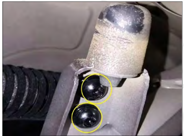
11. Close to the car body, fasten our tailgate bracket with bolts and nuts on the tailgate.
