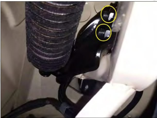
11. Close to the car body, fasten our tailgate bracket with bolts and nuts on the tailgate.
